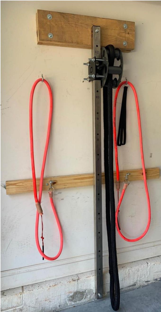
RX505 SECURED TO RAIL WITH BACKPLATE
