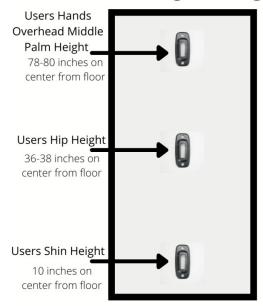
**Step 5:** Next, place the Mounting Trax at the desired height and mark with a pencil, in between the holes of the Mounting Trax, where you need to drill your pilot holes before you screw in the lag screws.
